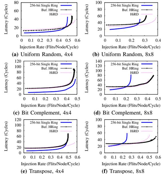
Fig. 8: Synthetic-traffic evaluations for 4x4 and 8x8 networks.
