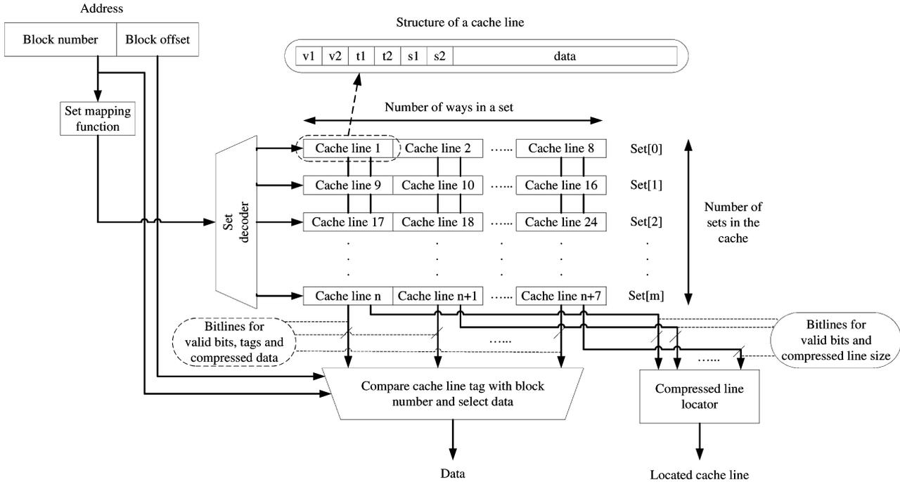
Fig. 4. Structure of a pair-matching based cache.
