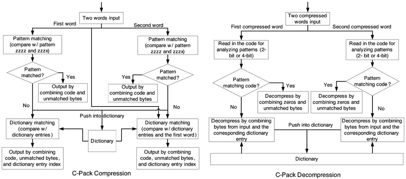
Fig. 2. C-Pack (a) compression and (b) decompression.
