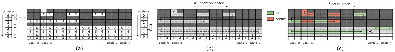
Fig. 6: The diagrams show how we can force the buddy allocator into providing us with contiguous physical memory and how we can detect this contiguous areas using our *hit*-pattern. (a) shows the buddy allocator keeping track of available memory in its *free\_lists*. (b) shows the process of allocating 2 arrays namely *a* and *b* of respectively 15 and 40 pages, and the result of this process on the buddy’s *free\_lists*. (c) shows how our *hit*-pattern detects the contiguous memory backing *b*.
