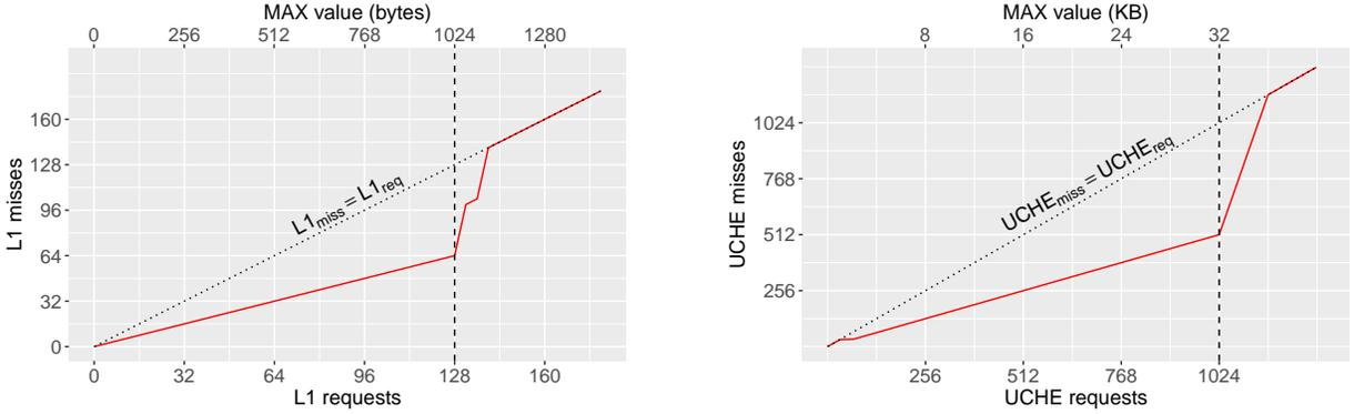
Fig. 3: Cache *misses* over cache *requests* for L1 and UCHE caches. The results are extracted using the GPU performance counter after each run of the shader in Listing 1 with STRIDE equal to cacheline size and increasing MAX value.
