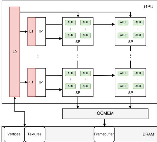
Fig. 2: Building blocks of an integrated GPU
