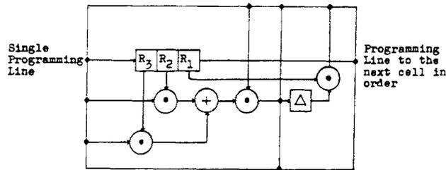
Fig. 8. A linear select programmable cell structure.
