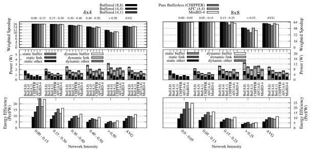
Figure 3. Performance (weighted speedup), network power, and energy efficiency (performance per watt) in 16 (4x4) and 64 (8x8)-node CMP systems.
