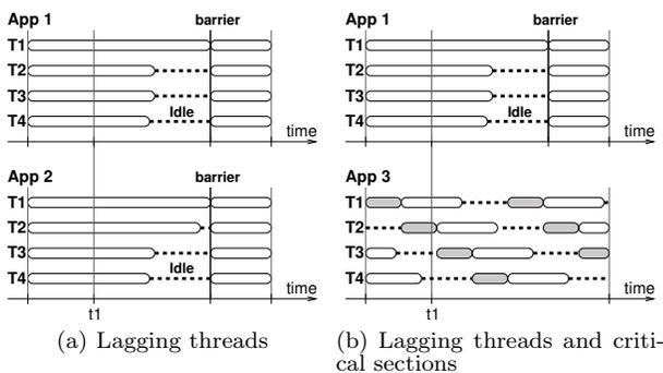
Figure 3: Examples of lagging threads and critical sections.
