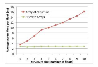
The green line is the time for a kernel that accesses an array that is stored as discrete sub-arrays, that is, all i-th members of all array elements are stored in the i-th sub-array, in consecutive memory locations. The red line is the kernel time with an array that contains members of the same structure in consecutive memory locations.
