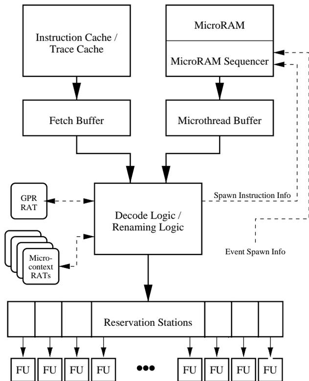
**Figure 2. High-level block diagram of an SSMT machine.**
