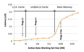
Figure 3. Latency measurement of the designed micro-benchmarks with varying active data working set sizes.
