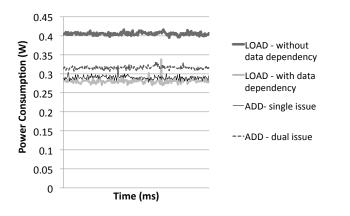
Figure 1. Dynamic power consumption comparison for benchmarks that perform continuous load instruction execution with and without data dependency, and add instruction execution utilizing one or both pipelines of the dual-issue ARM Cortex-A9 processor.
