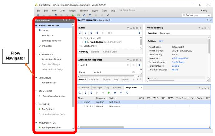
On the left side of Vivado, you will find the "Flow Navigator", which you will extensively use to develop your project and finally program it to the FPGA board.
