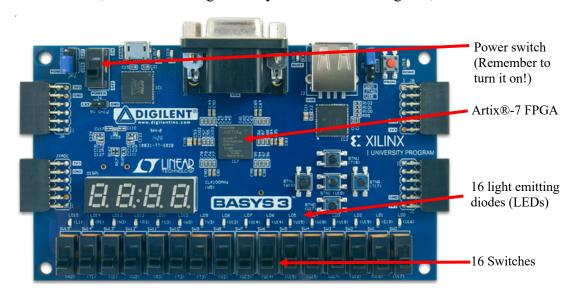
This board includes an Artix®-7 FPGA chip which we can program, some switches, some light-emitting diodes (LEDs), and some other cool features. You can learn more about the Basys 3 Starter Board from:
