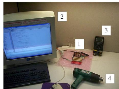
**Figure 1. Experimental setup for testing page retention times.**
