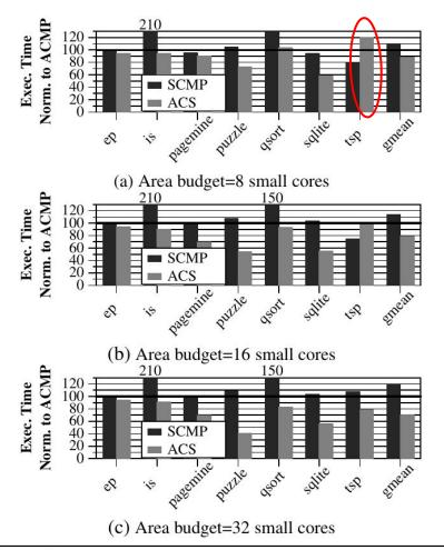
**Figure 8.** Execution time of workloads with coarse-grained locking on ACS and SCMP normalized to ACMP
