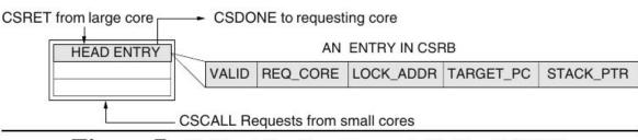
Figure 7. Critical Section Request Buffer (CSRB)
