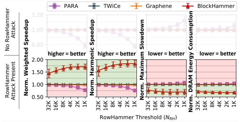
BlockHammer has significantly better performance and lower energy consumption as RH worsens (when attack is present) as
