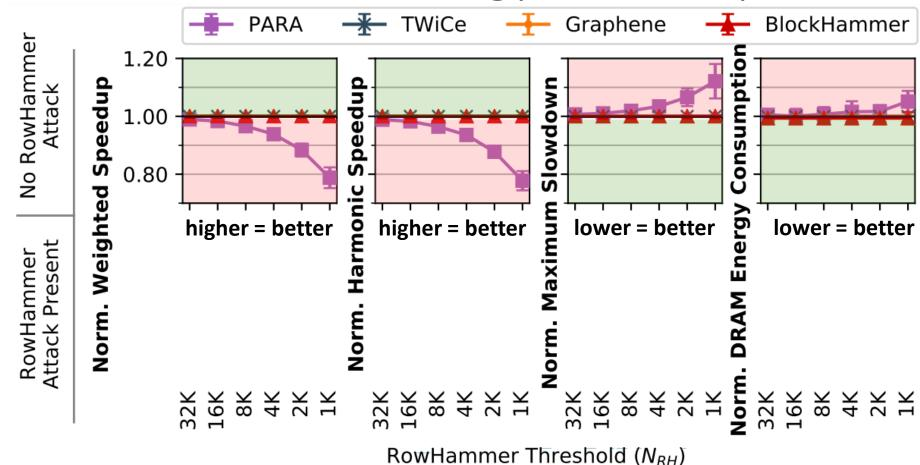
BlockHammer has negligible performance and energy consumption overheads and still does if RH worsens (when no attack is present)
