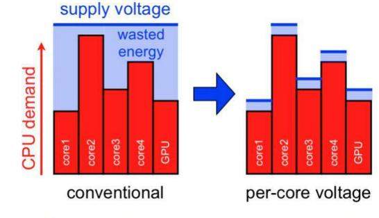
Figure 1. Per-core DVFS can reduce wasted energy due to shared supply voltages.
