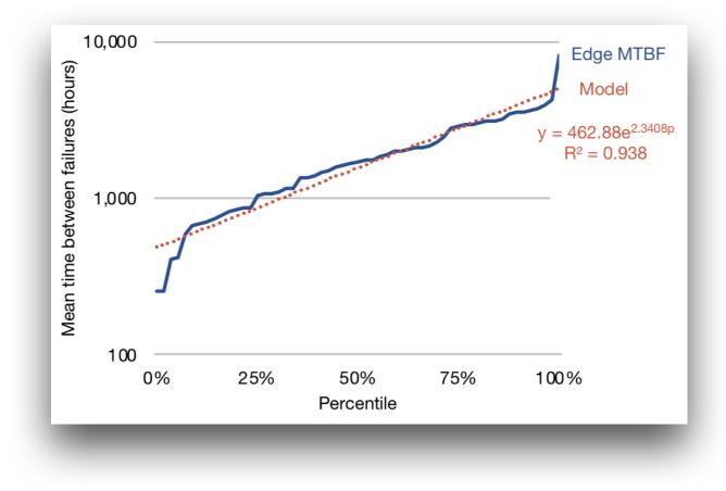
Typical edge node failure is in the order of months
