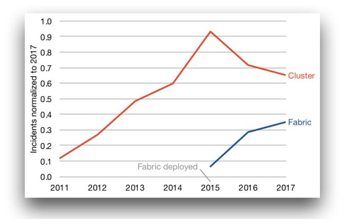
Cluster have 2x total incidents & 2.8x on a per-device level compared to fabric design
