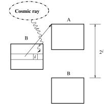
If  $2^i$  is larger than the object size, then  $x \oplus 2^i$  is likely to point to the base of a B object ( $\oplus$  is the exclusive-or operator):
