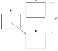
Thus, there's a field whose static type is A but which actually points to a B object; this can be exploited, as we will explain. On the other hand, suppose  $2^i$  is smaller than the object size; then the mutated field points within the A object:
