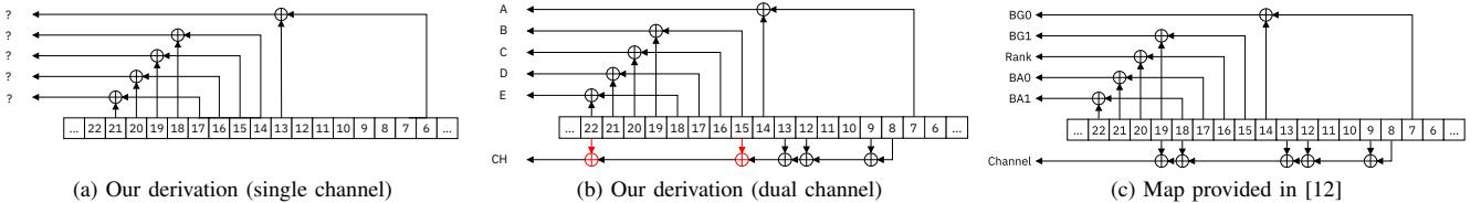
Figure 4: Skylake map functions derived by us for single channel (a) and dual channel (b) memory configurations, and from [12]
