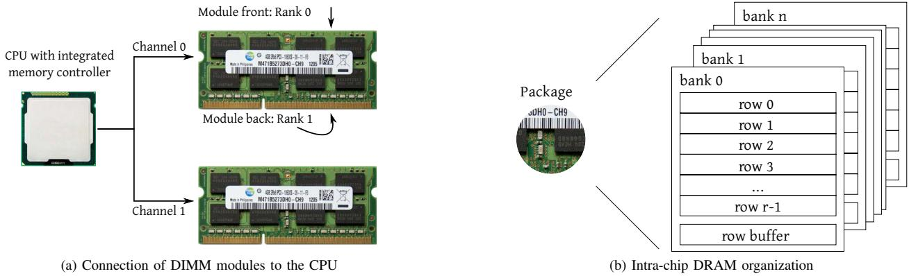
Figure 1: Depiction of hierarchy of the components in a modern DRAM subsystem
