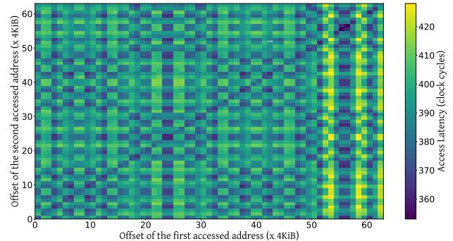
Figure 2: Access latency heatmap of our Skylake platform, derived applying the method in [7]
