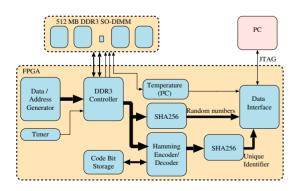
Fig. 3. Block diagram of the experimental DRAM PUF circuit.
