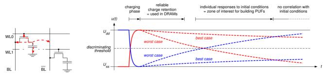
Fig. 1.1 Possible leakage paths of Fig. 1.2 Charge decay of an initially charged capacitor over time. a DRAM cell
