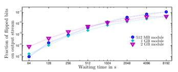
Fig. 4. Bit stability at increasing waiting time
