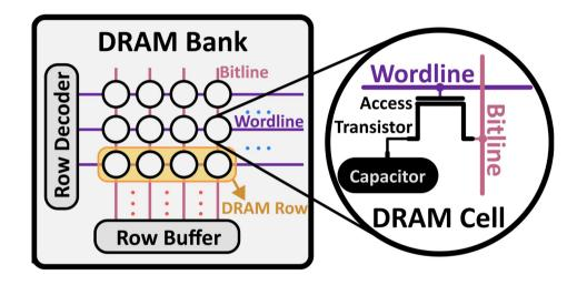
Note that the capacitor state must be restored after a row activation.
