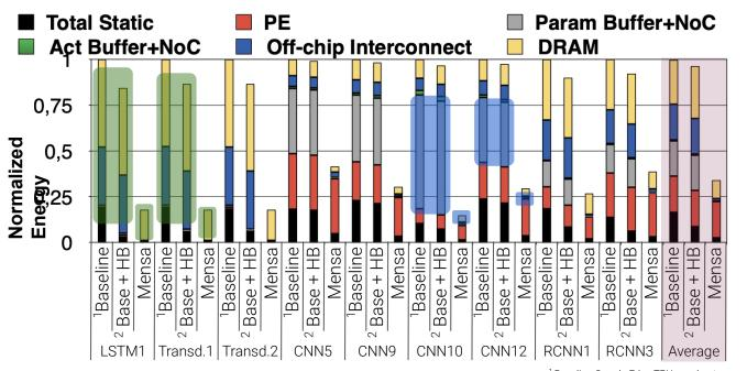
15.3x lower on-chip/off-chip parameter traffic energy by scheduling on accelerator with appropriate dataflow and memory bandwidth
