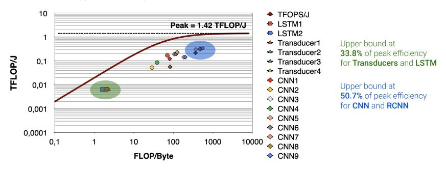
The Edge TPU provides only 37% of its peak energy efficiency, averaged across all models.
