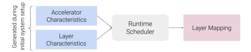
Mensa's software runtime scheduler determines on which accelerator each layer should run.
