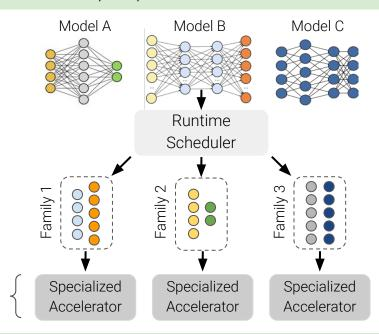
Mensa exploits the variations between and within layers for high efficiency and high performance.
