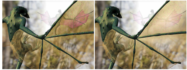
Figure 15: Transparency without and with pre-resolve effects: the left image sorts the geometry and resolves before applying a fog patch. The right image applies the fog patch to the translucent surfaces and then resolves. The fog is visible through the wing in the right image, but not in the left image. (Dragon models designed and created by Jeffery A. Williams and Glen Lewis.)
