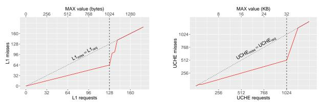
Fig. 3: Cache *misses* over cache *requests* for L1 and UCHE caches. The results are extracted using the GPU performance counter after each run of the shader in Listing 1 with STRIDE equal to cacheline size and increasing MAX value.
