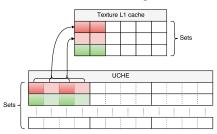
Fig. 4: Mapping of a 64-byte UCHE cacheline into multiple L1 cacheline over two different L1 sets.
