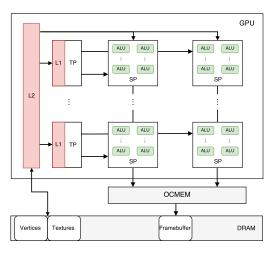
Fig. 2: Building blocks of an integrated GPU
