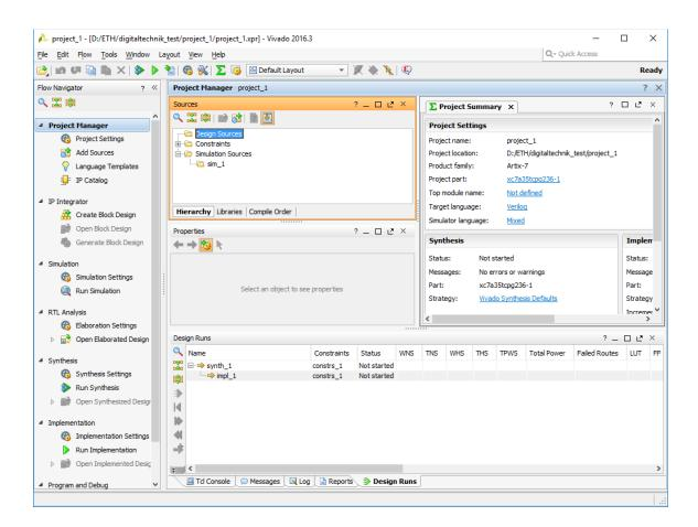
On the left side of Vivado, you will find the "Flow Navigator" which you will extensively use to develop your project and finally program it to the FPGA board.
