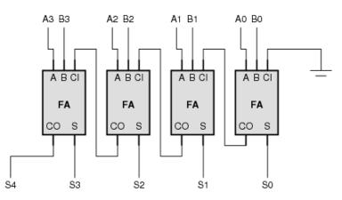
In the description (and the figure) the organization is so that the least significant bit is on the right and the most significant bit is on the left. This is partly for didactic purposes; the organization mimics the way we write numbers on paper.
