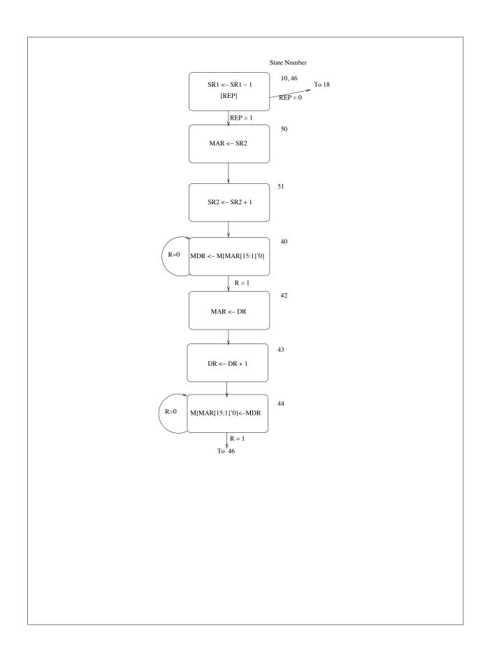
2. Add to the LC-3b datapath any additional structures and any additional control signals needed to implement REPMOVSB. Clearly label your additional control signals with descriptive names. Describe what value each control signal would take to control the datapath in a particular way.
