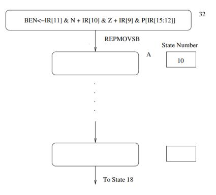
2. Add to the LC-3b datapath any additional structures and any additional control signals needed to implement REPMOVSB. Clearly label your additional control signals with descriptive names. Describe what value each control signal would take to control the datapath in a particular way.
