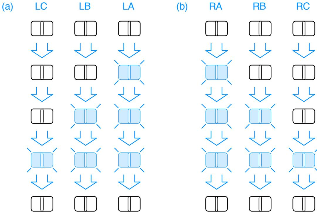
Figure 2. Flashing Sequence (shaded lights are illuminated)
