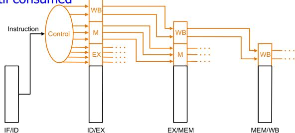
⇒ Option 2: carry relevant "instruction word/field" down the pipeline and decode locally within each or in a previous stage
