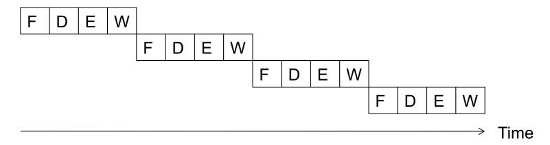
Pipelined: 4 cycles per 4 instructions (steady state)
