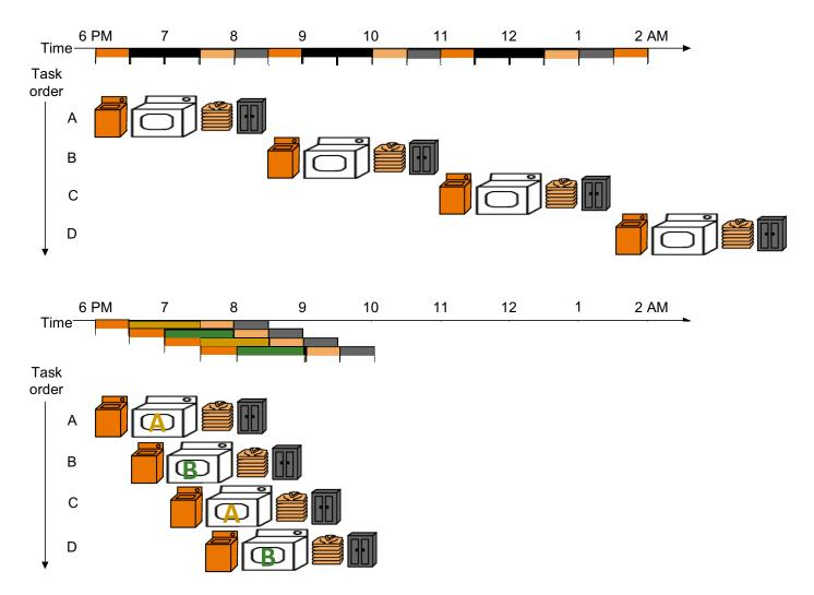
throughput restored (2 loads per hour) using 2 dryers
