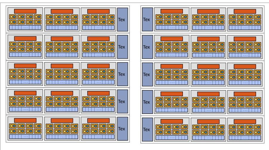
30 cores on the GTX 285: 30,720 threads
