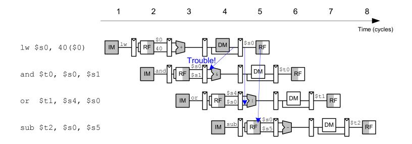
The **lw** instruction *does not finish* reading data until the end of the Memory stage, so its result *cannot be forwarded* to the Execute stage of the next instruction.
