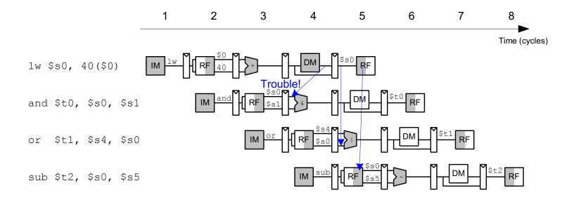
The 1w instruction has a two-cycle latency, therefore a dependent instruction cannot use its result until two cycles later.
