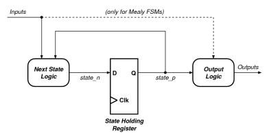
Figure 3. A simple view of an FSM.
