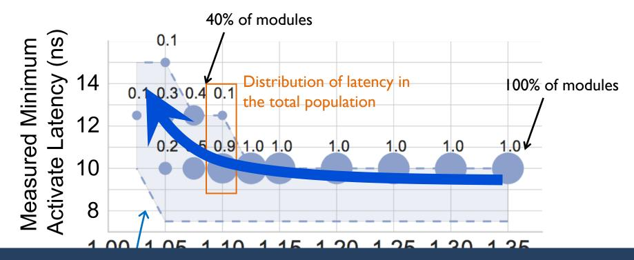
DRAM requires longer latency to access data without errors at lower voltage
