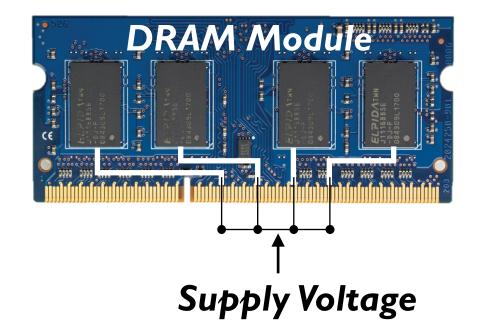
Adjust the supply voltage to every chip on the same module
