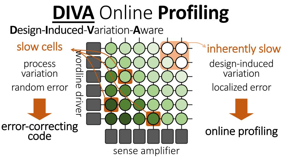
Combine error-correcting codes & online profiling → Reliably reduce DRAM latency
