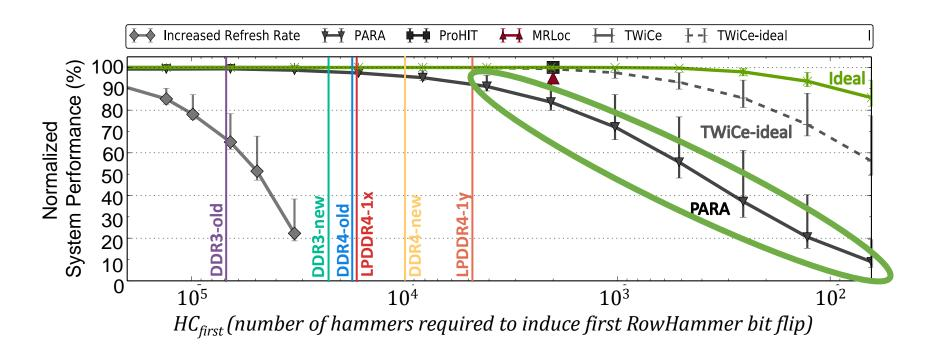
Only PARA's design scales to low HC<sub>first</sub> values but has very low normalized system performance
