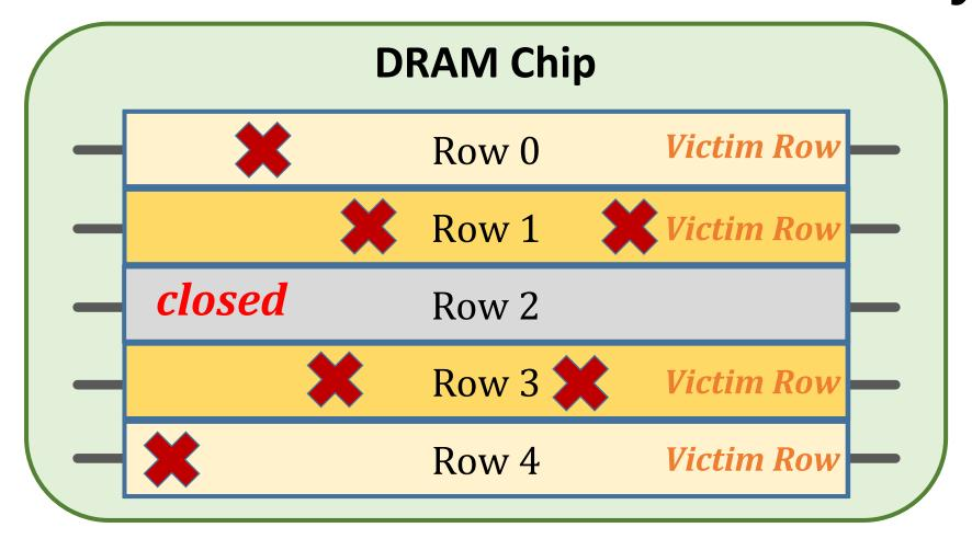
Repeatedly **opening** (activating) and **closing** (precharging) a DRAM row causes **RowHammer bit flips** in nearby cells
