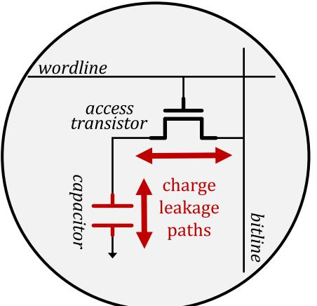
Stored data is **corrupted** if too much charge leaks (i.e., the capacitor voltage degrades too much) SAFARI
