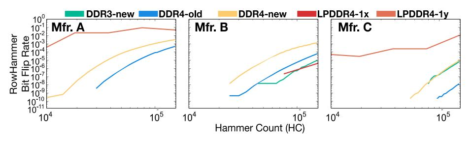
RowHammer bit flip rates **increase** when going **from old to new** DDR4 technology node generations
