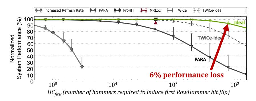
Ideal mechanism issues a refresh command to a row only right before the row can potentially experience a RowHammer bit flip
