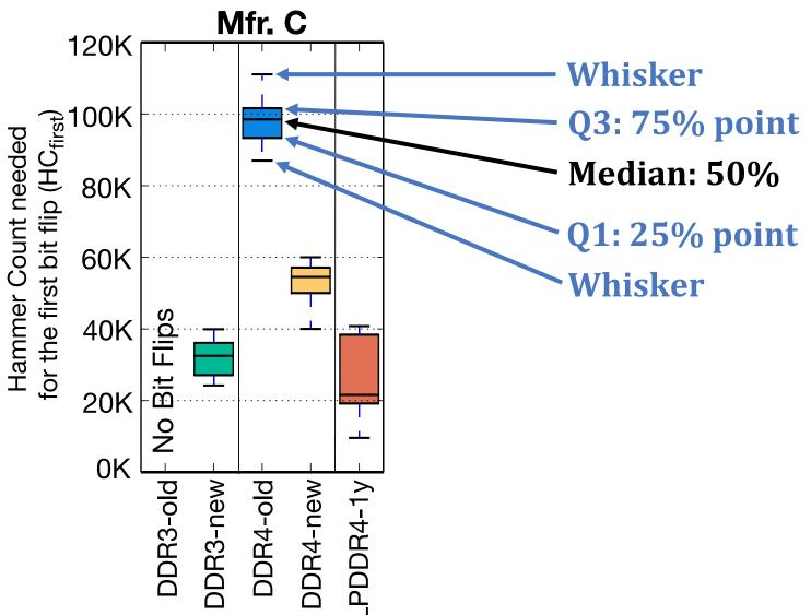
What is the minimum Hammer Count required to cause bit flips  $(HC_{first})$ ?
