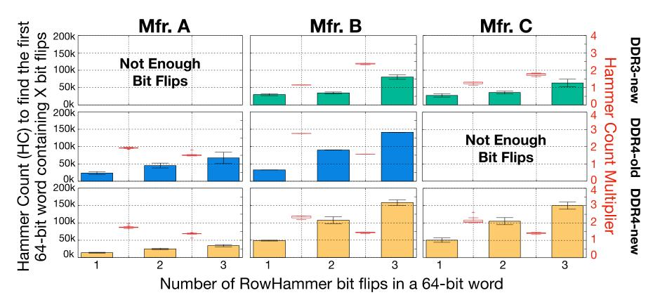
Single-error correcting code can improve HC<sub>first</sub> by up to 2.78× in DDR4 DRAM chips, and 1.65× in DDR3-new DRAM chips.
