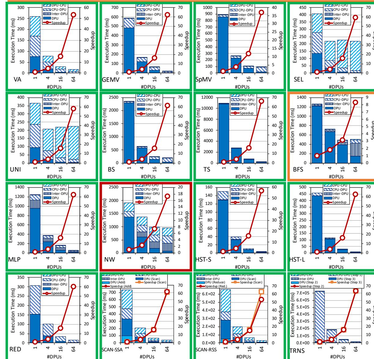
VA, GEMV, SpMV, SEL, UNI, BS, TS, MLP, HST-S, HSTS-L, RED, SCAN-SSA (both kernel), SCAN-RSS (both kernels), and TRNS (both kernels) scale linearly with the number of DPUs
