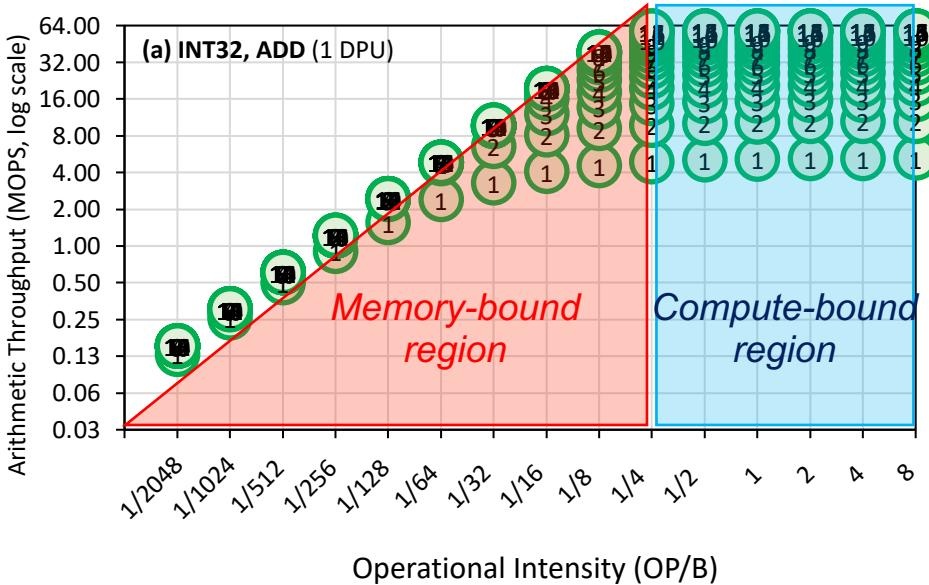
The throughput saturation point is as low as  $\frac{1}{4}$  OP/B,
