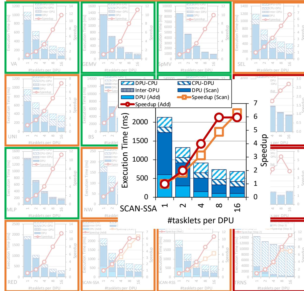
SCAN-SSA (Add kernel) is **not compute-intensive**. Thus, performance saturates with less than 11 tasklets (recall STREAM ADD).
